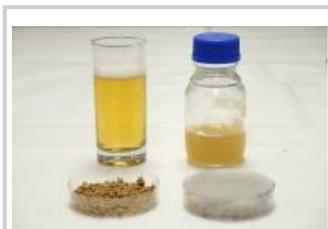
(Anticlockwise from bottom left) These are spent beer grains, fermented beer grains, nutrient liquid used to grow yeast, beer. Credit: NTU Singapore
